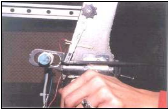
Figure 1. Placement of the CRT measurement device on the bow handle.
